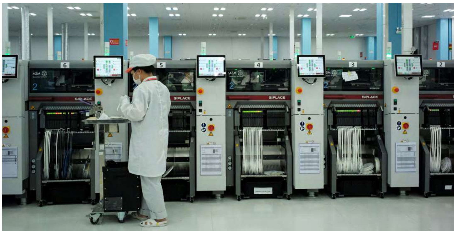
A worker checks the SMT process to produce ventilators at Vsmart factory of Vingroup, Hanoi, Vietnam 3 August 2020.
